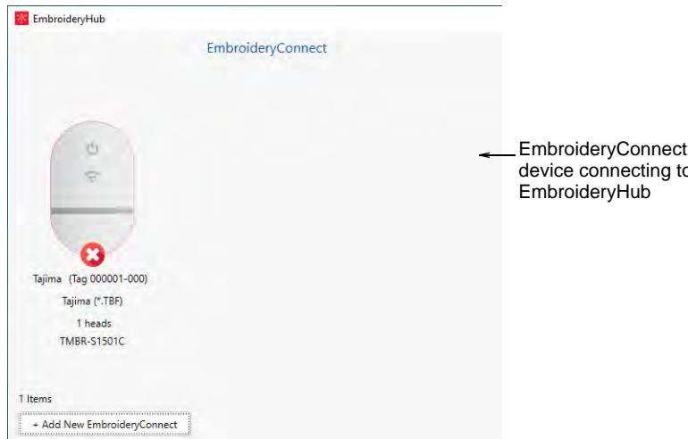
**10** Wait for the EC device to connect to the network and EmbroideryHub. The blue WiFi LED will flash and then turn solid blue when it has successfully connected.
