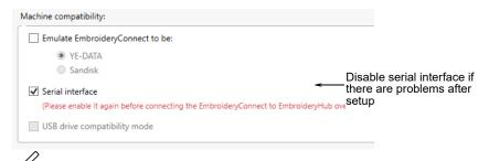
**Note:** If you turn off the serial interface and subsequently lose WiFi connection to the EC device, the only way to reconfigure it is to perform a 'hard reset'. See EmbroideryConnect troubleshooting for details.
